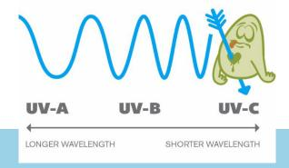
The germicidal effect of UVC radiation has the highest efficacy at a wavelength of 253, 7 nm (nanometers). This particular characteristic is mainly due to the destructive effect of UVC radiation on the DNA of germs. In particular, their reproductive system is damaged, preventing their growth and multiplication.
